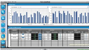
The Vertex GUI displays real-time information regarding channel power with respect to fading. This instantaneous display enables quick detection of deviations from expected behavior and the ability to efficiently debug problems.
