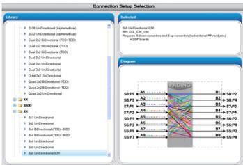
The GUI provides an easy-to-read display for high-channel density features that can be complicated to set up. For example, the connection setup for an 8x8 MIMO application, or 64 radio links, can be easily viewed using the pre-loaded option from the Connection Setup library.
