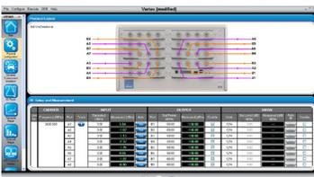
The cable connection diagram built-in to the Vertex GUI presents the actual cabling connections that need to be made. This feature makes it easy to cable complicated connection setups and minimizes cabling error. The image shown is the cabling setup for an 8x8 unidirectional configuration.
